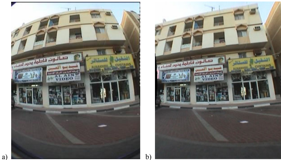
Figure 7: Barrel Distortion Correction using digital filters and image processing software. a) before correction, b) after correction.
