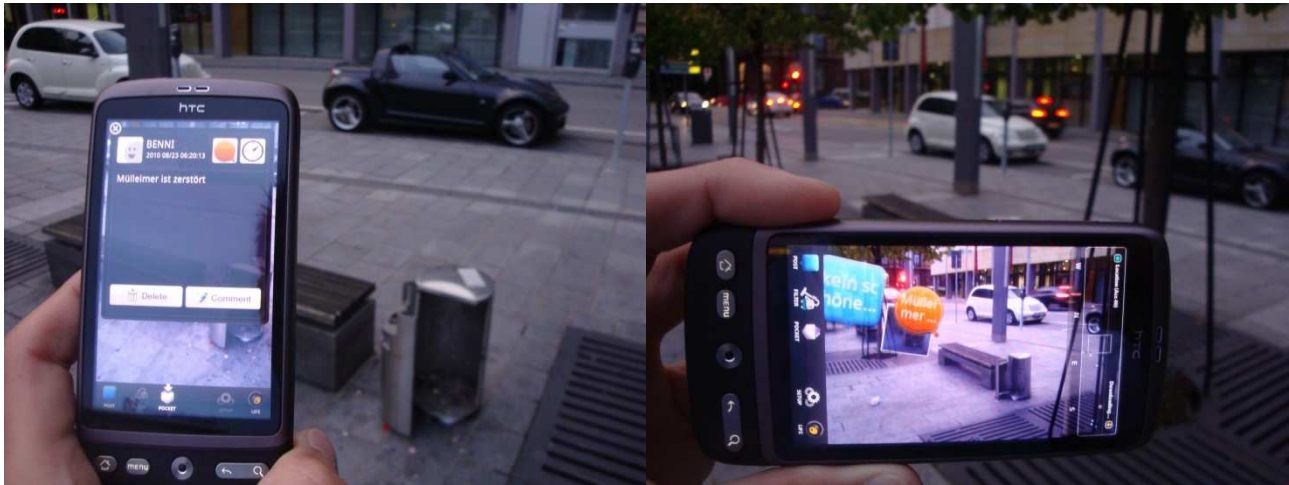
Fig. 5: Tagging 3D damage information by using SEKAI
