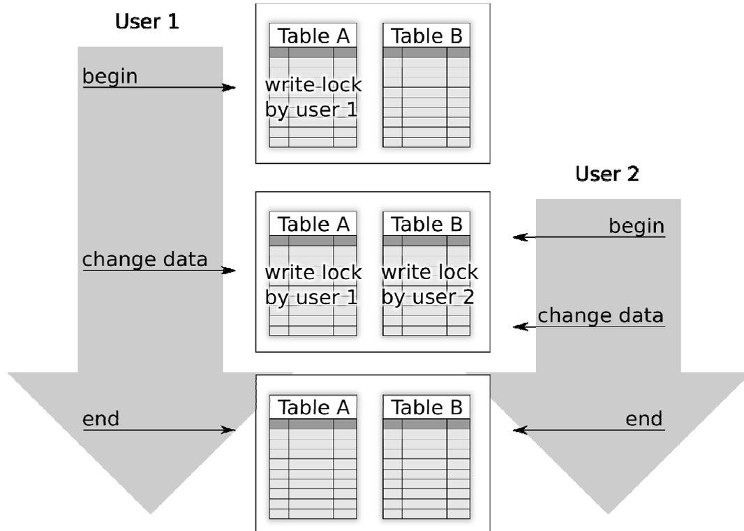
Fig. 2: The transactional locking of a RDBMS
