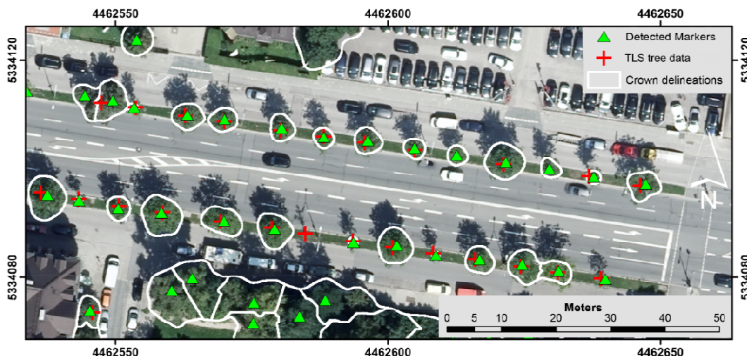
Figure 4: Visual comparison of markers from LM filtering and tree crowns based on MCWS with TLS tree positions. Aerial imagery is provided by Geobasisdaten© Landeshauptstadt München - Kommunalreferat - GeodatenService 2021.
